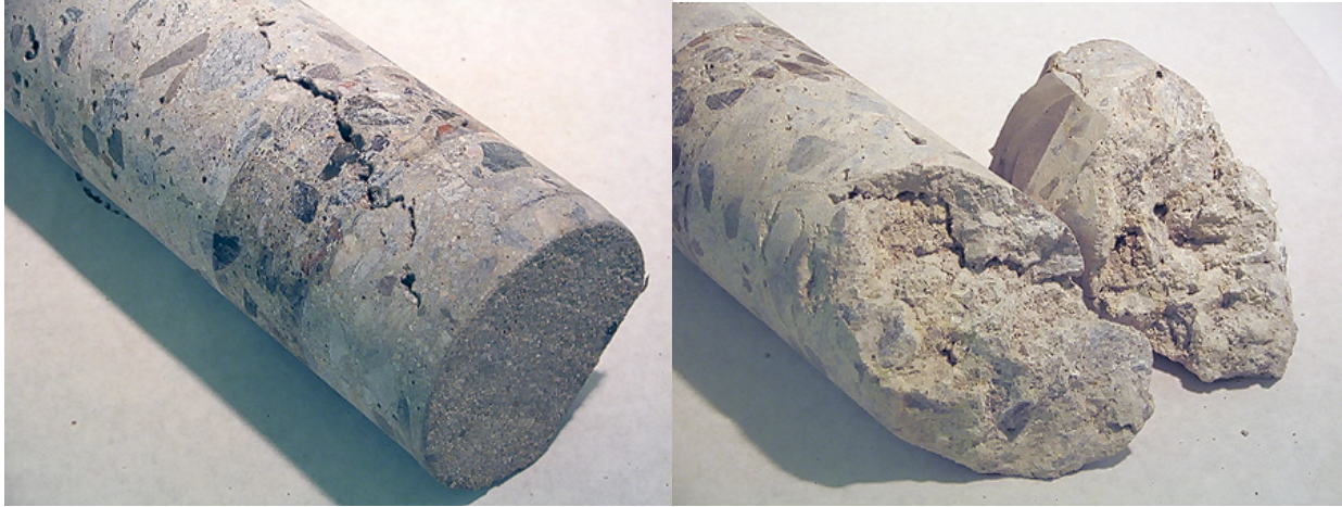
FIGURE 60. CLOSE-UP IMAGES OF IRREGULAR VOIDS, CORE A ON LEFT, CORE G ON RIGHT
